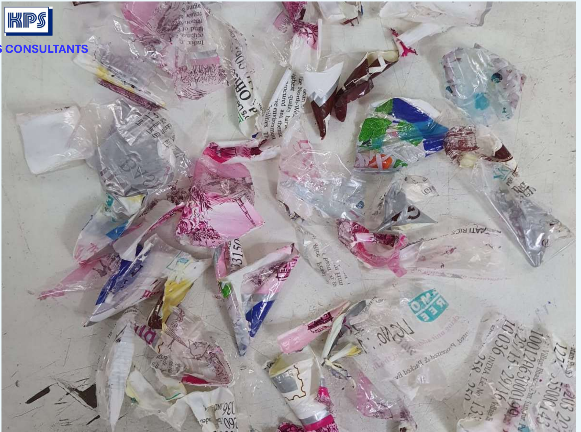
DE-LAMINATED FILM AFTER TREATMENT (LAB SCALE)
