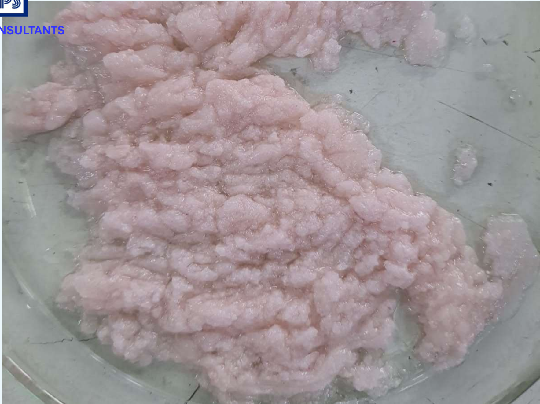
SEPERATED PE FRACTION ALONG WITH GUMMY TIE LAYER MATERIALS (later washed with water to remove the colour)
